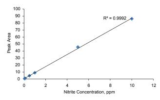
Fig. 2: Calibration Curve for Nitrite 0.05-10 ppm range
