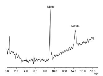
Fig. 3 Chromatogram of  $0.05\,\mathrm{ppm}$  Nitrite and 0.05 Nitrate solution.
