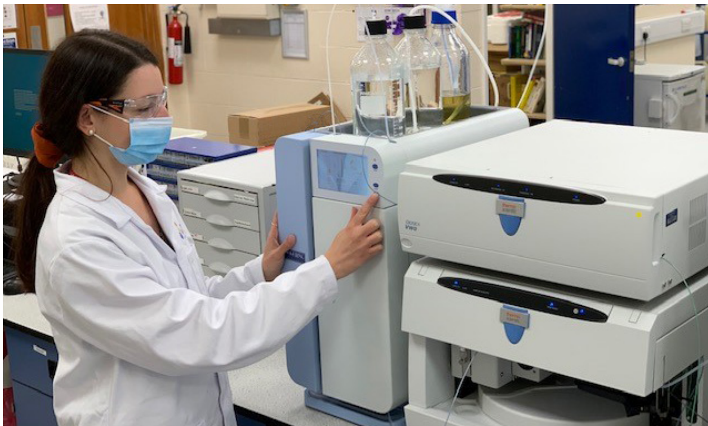
A scientist checks the Pinnacle PCX post-column derivatization instrument. Image courtesy of Reading Scientific Services Ltd (RSSL).
