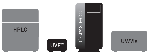
Flow diagram for NDELA analysis according to DIN EN ISO 10130:2009
